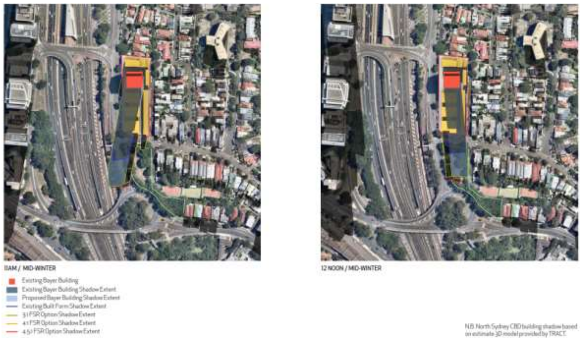
Figure 7. Shadow Analysis Extracts (11 am – 12 pm Mid-Winter) – Alfred Street Massing Study (Source: AJ+C, 2021)
